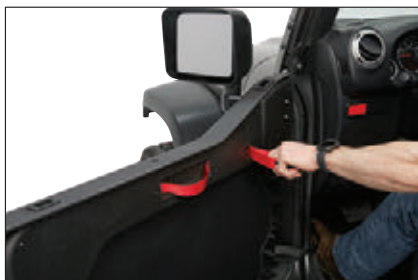
Remote latch release and OEM-quality check strap
