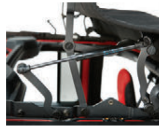
Gas assist struts help in raising and lowering the top
