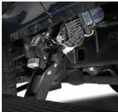
Powerboard Motor Detail
